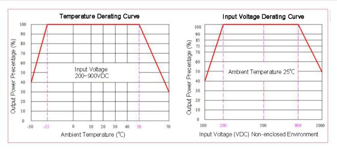
Note 1: The output power should be derated based on the input voltage derating curve at 100~200/900~1000VDC. Note 2: This product should operate at a natural air condition, please contact us if it need be used at a closed space.
