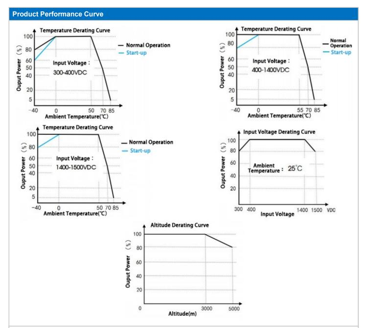
Note 1: The output power should be derated based on the input voltage derating curve at 300 to 400VDC / 1400 to 1500VDC.
