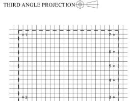
Unit:mm Printed board vertical view Grid:2.54mm(0.1inch) General tolerance:±0.5mm Pin tolerance:±0.10mm
