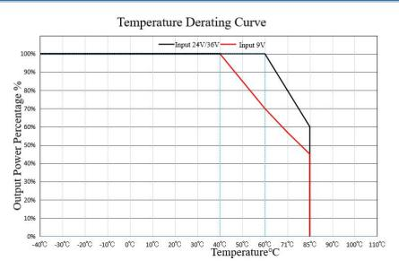
Note1: The temperature derating curve is based on the product with heatsink and no wind environment.
