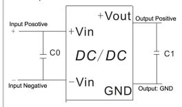
2. Input reflecting ripple current test circuit:
