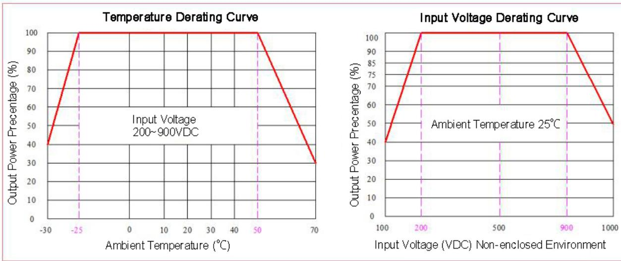
Note 1: The output power should be derated based on the input voltage derating curve at 100~200/900~1000VDC.
