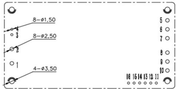
Recommended PCB holes size
