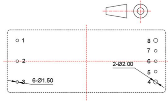
Recommended holes size for PCB layout
