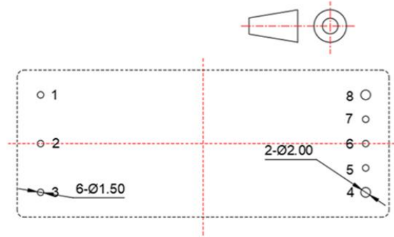
Recommended holes size for PCB layout
